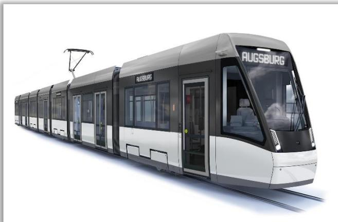
The seven-part unidirectional trains enter into service on the lines of Bavaria's second largest tram system from 2022 onwards. The fully low-floor accessible and barrier-free vehicles are 42 meters long and can
