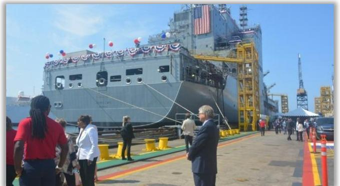
Provided by Inmar Systems, on board are 21 Type D Straight Line wipers and 100 series controllers. The Lewis-class will be able to carry 160,000 barrels of fuel to support carrier strike group operations. Like the Kaiser-class, the Lewis-class oilers have fine lines for tank vessels, and they will be capable of making up to 20 knots.
