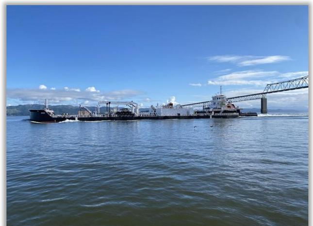
The ATB is specially designed to add efficiency and range to transport clean petroleum products for Crowley Fuels, the company's Alaska-based business unit. It has a design speed of 9 knots.
