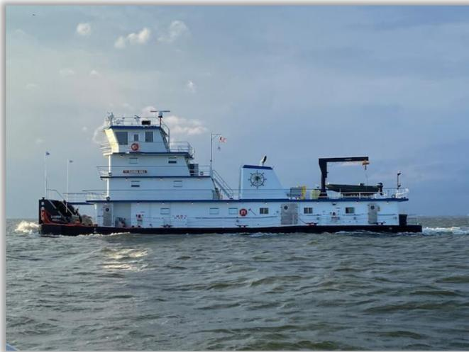
The vessel's twin Caterpillar marine diesel engines deliver over 2,000 hp each and turn 100"x69" stainless steel propellers through Twin Disc reverse reduction gears with a 6.56:1 ratio. Sleeping accommodations and facilities have been provided for a nine-person crew.
