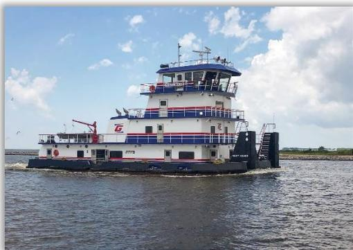
The mv. Rusty Moore is a 2,400 hp., open-wheel, triple-screw towboat that measures 94 by 34 by 10.75 feet. The hull models our 2,800 hp. class boats and uses the same rudders and tail shafts, reducing the need for spares.
