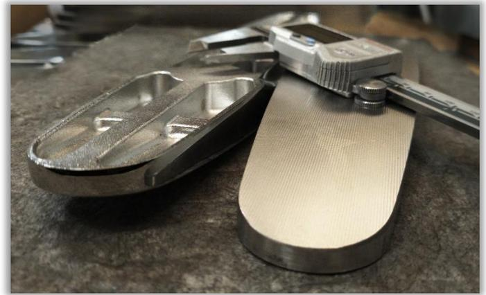
First, we sculpt all unnecessary metal out of the main components, reducing the weight of each cleat by approximately 30%. Then, to still be able to achieve the renowned Monitor Marine finish, each of the cleat components get CNC machined and then polished to a jewellery-like standard.
