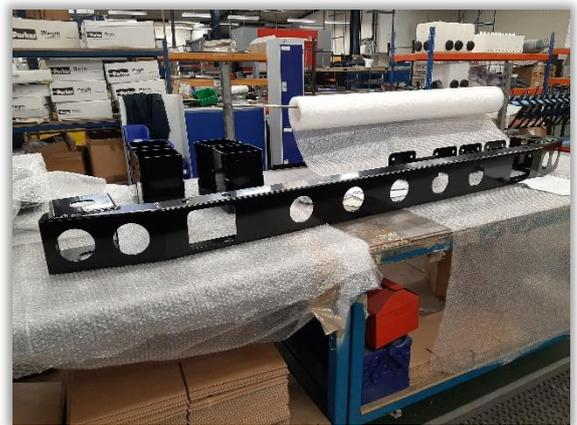
Laser cutting, saw cutting, machining, coded welding, and zinc-plating, all done in less than 2 weeks for a brand-new assembly.
