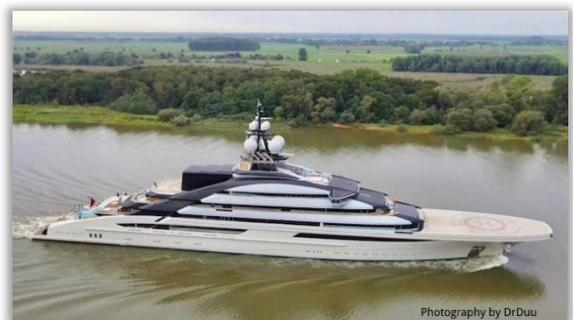
The vessel has two helicopter decks, suitable for some of the largest civilian helicopters. The aft deck features an integrated retractable hangar, and both helidecks incorporate MMI’s new flange-mounted 7516 tie-downs.
