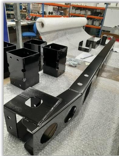
The Rail client had an extremely short lead time requirement. They needed to move a train during build and required a drawbar to do so. Subsequently, we were given the task of manufacturing a drawbar & mounting structure with a deadline of 12 days.
