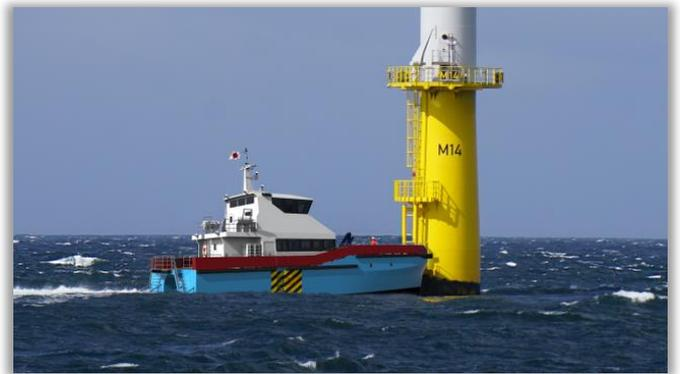
Destined for duty in the Akita Prefecture region of Japan, the two vessels have been designed specifically for operations and maintenance of the Akita and Noshiro offshore wind farms, the first utility-scale offshore wind project in Japan.
