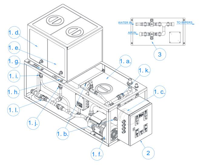
The Window Wash System consists of a galvanised steel frame enclosing all containers, pipe work, valves and electrical controls required to provide a window washing function. The complete frame may be mounted to the deck.
