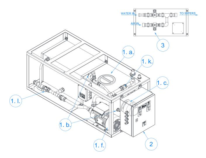
The Window Wash System consists of a galvanised steel frame enclosing all containers, pipe work, valves and electrical controls required to provide a window washing function. The complete frame may be mounted to the deck.
